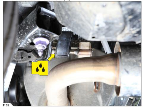
INSTALLATION TIP: for easier removal, lubricate the original rubber brackets (WD40<sup>®</sup>)\*.
