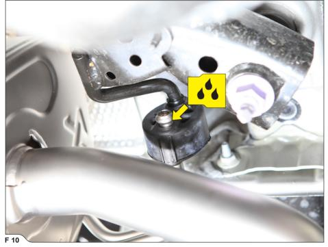
INSTALLATION TIP: for easier mounting, lubricate the original rubber bracket (WD40<sup>®</sup>)\*
