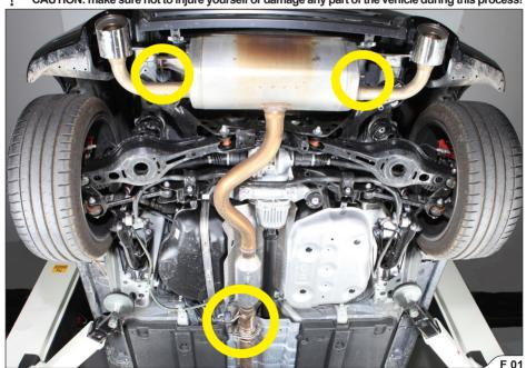
INSTALLATION TIP: for easier removal, lubricate the original rubber brackets (WD40<sup>®</sup>)\*.
