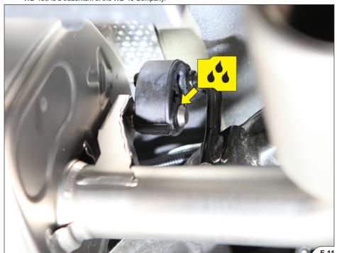
INSTALLATION TIP: for easier mounting, lubricate the original rubber brackets (WD40<sup>®</sup>)\*.
